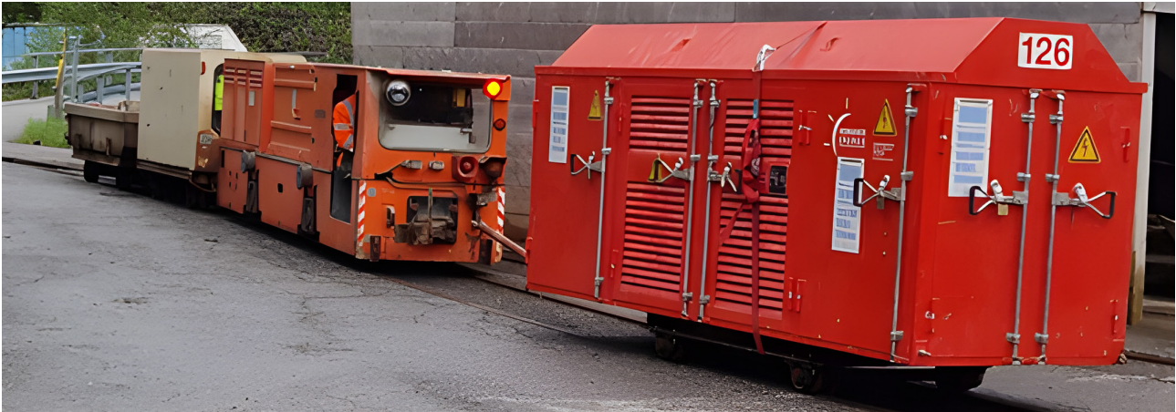
8 MV/LV Transformer cab before gallery entrance
