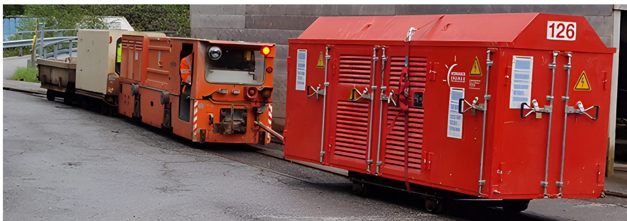
8 MV/LV Transformer cab before gallery entrance
